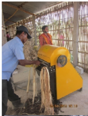
Old Banana fibre extraction machine (Raspador) on the right
