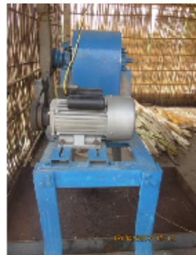
Improved Banana fibre extraction machine on the left
